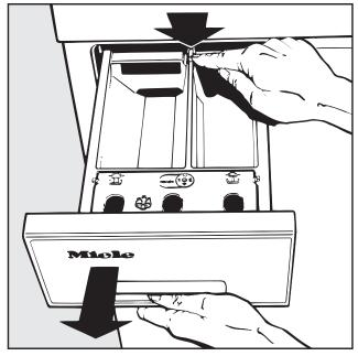
Press down the red release catch and at the same time pull the drawer right out of the machine.
