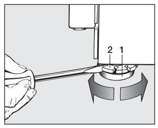
■ Hold the foot **1** firm using a pipe wrench and turn the counternut **2** to the right firmly up against the housing with a screwdriver.
